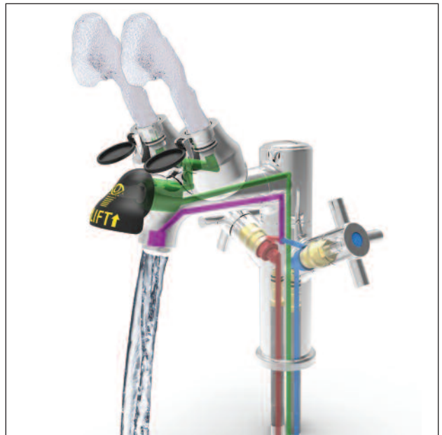
A safe dual-function unit has an independent plumbing supply to the eyewash function (green), which operates from its own activator handle without use of the faucet valves. The faucet valves get normal hot (red) and cold (blue) supply, which they mix in the faucet neck (purple). There is never a danger of scalding water being delivered to the eyes.
