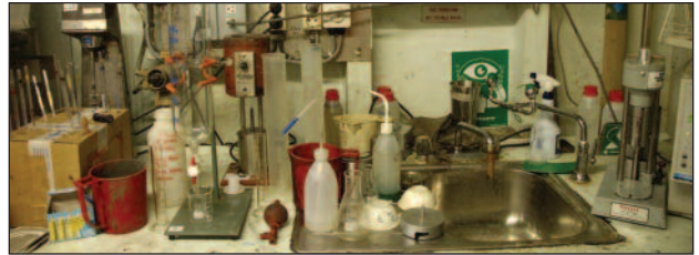
Eyewash stations are often badly marked, difficult to find and difficult to operate in a panicked state, causing them to fall short of the real safety goal of treating eye burns quickly.
